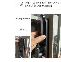
Note:1.Install battery first and then screen.2 Tight the screen to lock panel without chink
